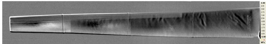
**Figure 5.** Stress distribution of the convex side of the wind blade.
