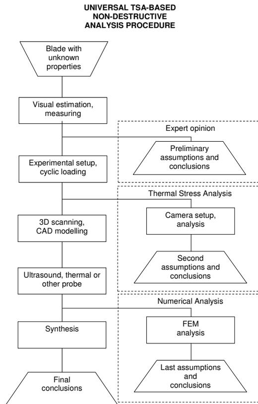
**Figure 14.** The scheme of a non-destructive analysis procedure based on the TSA, [7].
