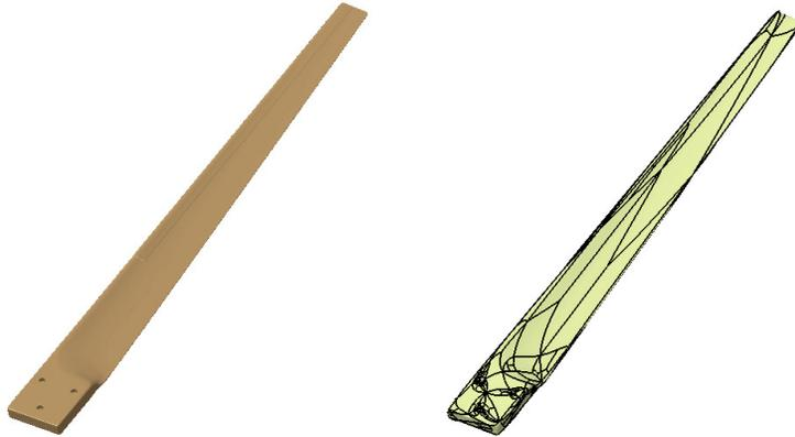
**Figure 8.** The scanned geometry and reconstructed CAD surface consisting of CAD patches.
