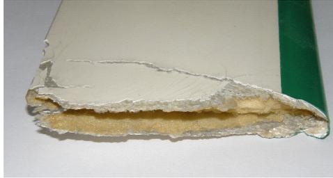
**Figure 2.** Ruptured wind turbine blade with structure shaped as airfoil (roving mantle), type b). The core is filled out with expanded polyurethane.
