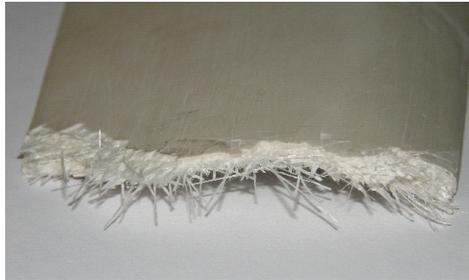
**Figure 3.** Ruptured wind turbine blade fully filled with fiberglass tapes randomly divided in polymer core, type c).
