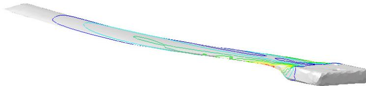
**Figure 13.** The stress distribution and maximal deformation for 2<sup>nd</sup> mode of vibrations.
