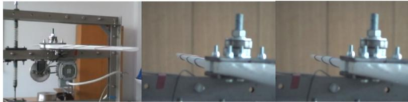
**Figure 4.** Experimental setup – load frame mechanism and blade vibrations for the 2nd mode.
