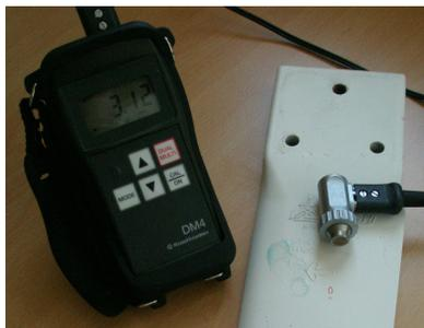
**Figure 9.** The ultrasonic thickness gauge measurement.
